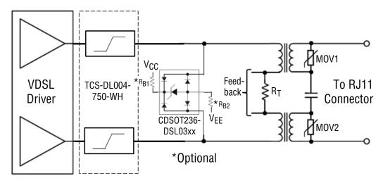
Figure 3. VDSL Driver Protection Design with Transient Current Suppressor Technology
