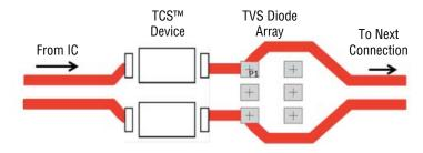
Figure 4. Connecting a Differential Signal to the Model CDSOT236-DSL03xx and TCS™ Device
