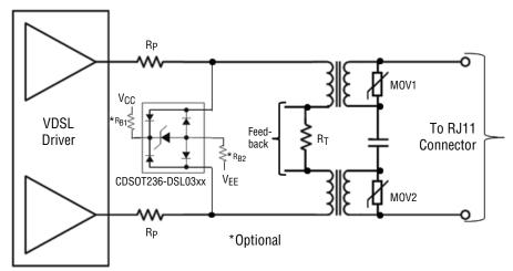
Figure 1. VDSL Driver Protection Design Topology
