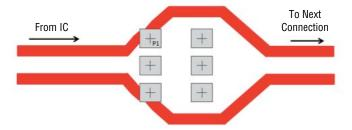
Figure 2. Connecting a Differential Signal to the Model CDSOT236-DSL03xx
